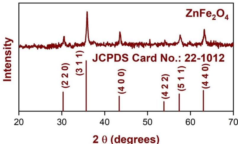
FIG. 1. XRD pattern of ZnFe<sub>2</sub>O<sub>4</sub>.
